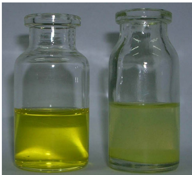
Fig. 1 Dispersivity of CdS nanoparticles in cyclohexane ( left ) and ethanol ( right )
